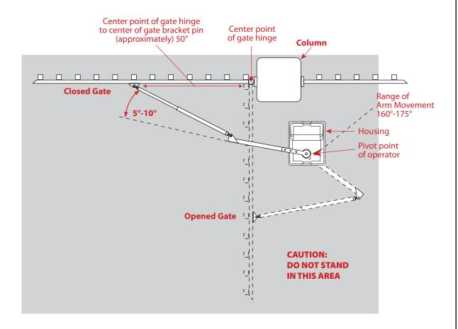
**IMPORTANT**: Be sure the operator housing will not be hit by a fully open gate and that the gate column will not interfere when housing is installed.
